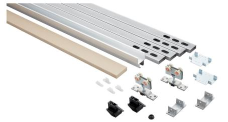
Each kit includes one CP-803 Header Track x length based on kit size, two CP-HB2X4 Header Brackets, two CP-830 Drywall Support x length based on kit size, four (or six) Steel Uprights x length based on kit size, two (or three) CP-2X4 Foot Brackets, two C-411 Quick Release Hangers, two CDC-411 Catch/Stops, set of C-1200 Guides and necessary fasteners
