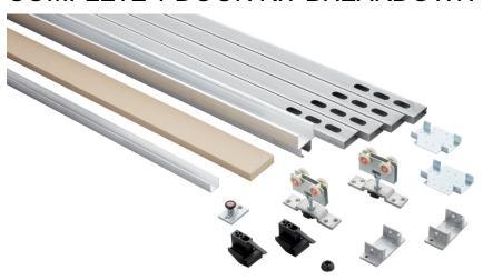
Each kit includes one CP-803 Header Track x length based on kit size, two CP-HB2X4 Header Brackets, two CP-830 Drywall Support x length based on kit size, four (or six) Steel Uprights x length based on kit size, two (or three) CP-2X4 Foot Brackets, two C-411 Quick Release Hangers, two CDC-411 Catch/Stops, one C-914 Guide Channel x length based on kit size, one CP-913 Pocket Guide and necessary fasteners
