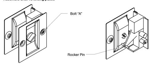
Plates can be reversed to match required orientation. Unscrew both bolts "A" to remove plates. Reverse and reattached. Be sure to engage fork arm with rocker pin before reinstalling bolts.
