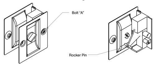
Plates can be reversed to match required orientation. Unscrew both bolts "A" to remove plates. Reverse and reattached. Be sure to engage fork arm with rocker pin before reinstalling bolts.
