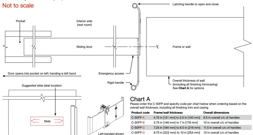
Note: The emergency access is also located on the exterior side next to the rigid handle.
