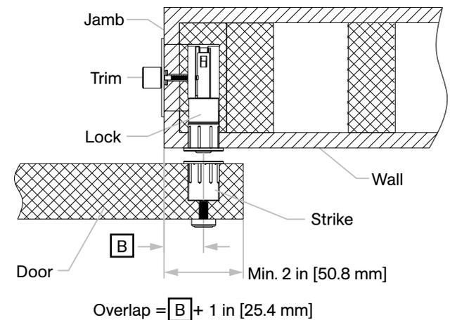
Template dimensions do not provide allowances for gaps between wall studs and drywall.
