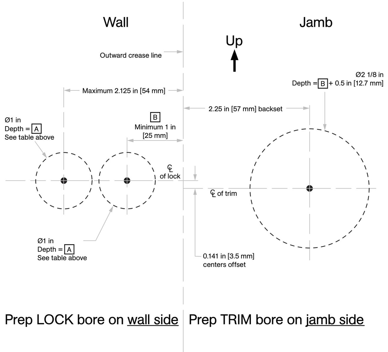
Template dimensions do not provide allowances for gaps between wall studs and drywall. Refer to installation instructions for more details.
