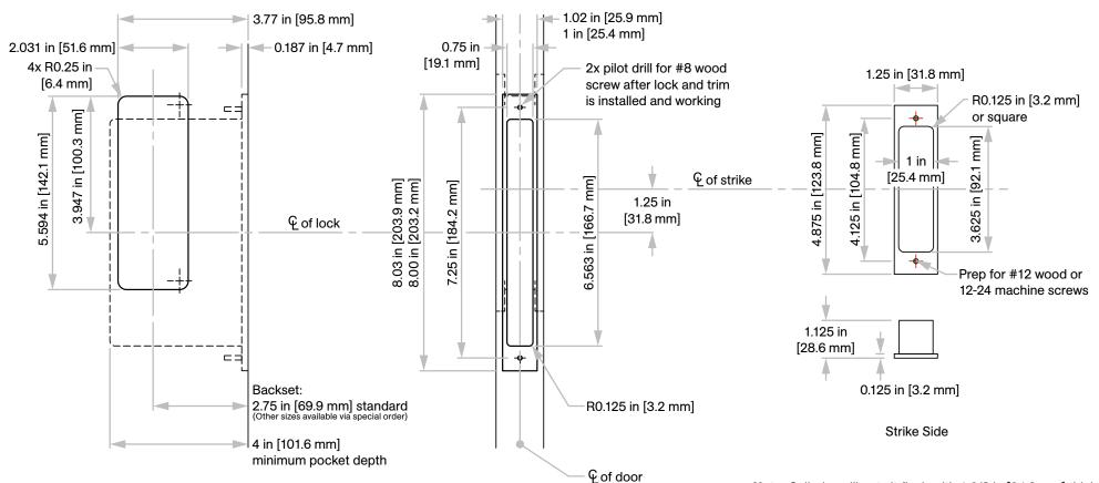
Note: Cylinder will not sit flush with 1 3/8 in [34.9 mm] thick doors.
