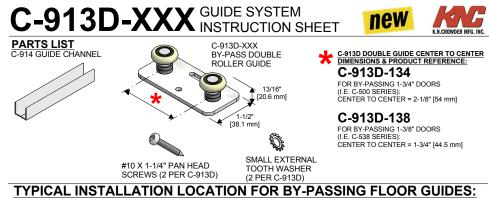
GUIDE CHANNEL IN DOOR WITH BY-PASSING GUIDE ON FLOOR
