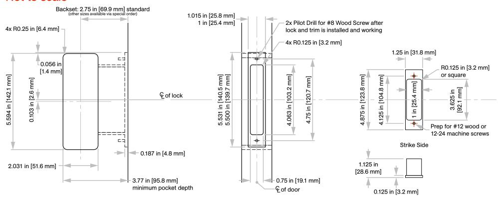
Note: When using two 1 in [25.4 mm] depth cylinders, they will not sit flush with flush pulls on a 1 3/4 in [44.5 mm] thick door therefore the cylinders will protrude past face of door.
