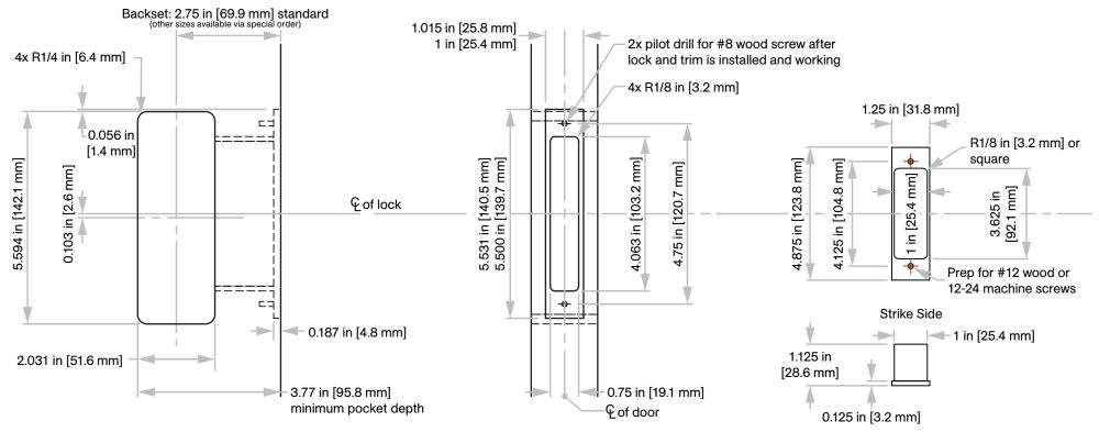
**Note:** Using two 1 in [25.4 mm] depth cylinders will not sit flush with flush pulls on a 1 3/4 in [44.5 mm] thick door; therefore, the cylinders will protrude past the face of the door.
