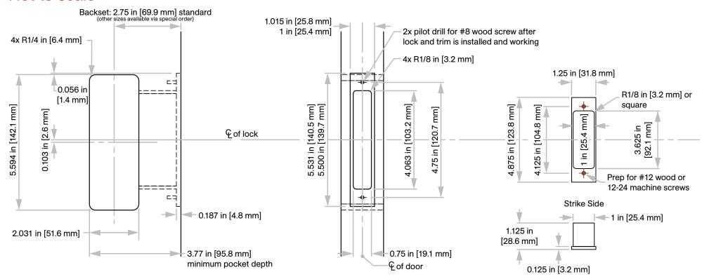
**Note:** Using two 1 in [25.4 mm] depth cylinders will **not** sit flush with flush pulls on a 1 3/4 in [44.5 mm] thick door; therefore, the cylinders will protrude past the face of the door.
