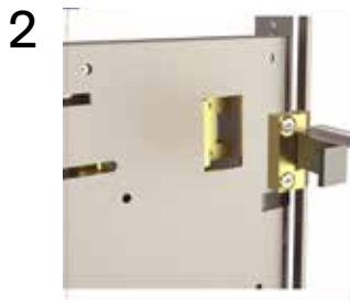
Remove Bolt from Lock Body Extend the bolt and loosen screws without removing them and remove bolt assembly from the lock
