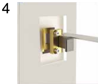
Reattach Bolt Slightly rotate loose thumb turn to make lock body screws visible Reinstall bolt assembly by aligning screw holes Tighten screws Use thumb turn to fit bolt assembly back in
