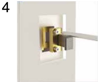
Reattach Bolt Slightly rotate loose thumb turn to make lock body screws visible Reinstall bolt assembly by aligning screw holes Tighten screws Use thumb turn to fit bolt assembly back in
