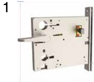
Expose Screws Rotate thumb turn 90 degrees to project bolt and expose the two bolt screws
