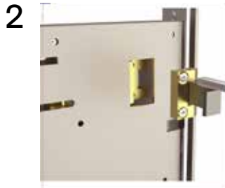
Remove Bolt from Lock Body Extend the bolt and loosen screws without removing them and remove bolt assembly from the lock
