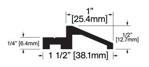
**Operation:** Build Any Size Threshold Features: Mill Finish Extruded Aluminum Application: Ideal for Residential, Commercial & Industrial Maximum Length: 156 in [3962 mm]
