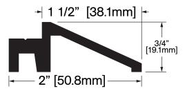
**Operation:** Build Any Size Threshold Features: Mill Finish Extruded Aluminum
