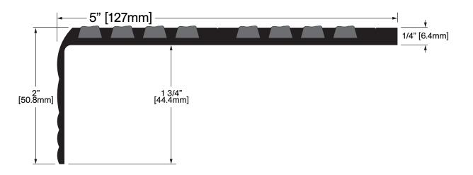
**Operation:** Stair Nosing Features: Mill Finish Extruded Aluminum with Aluminum Oxide Grit in Epoxy Base Application: Ideal for Residential, Commercial & Industrial Maximum Length: 216 in [5486 mm]
