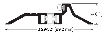
**Operation:** Thermal Break Threshold Features: Mill Finish Extruded Aluminum with Neoprene Insert included Application: Ideal for Residential, Commercial & Industrial Maximum Length: 192 in [4877 mm]
