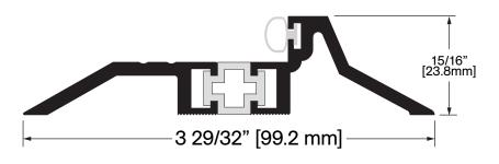
**Operation:** Thermal Break Threshold Features: Mill Finish Extruded Aluminum with Silicone Insert included Application: Ideal for Residential, Commercial & Industrial Maximum Length: 192 in [4877 mm]
