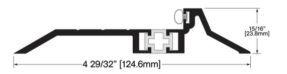
**Operation:** Thermal Break Threshold Features: Mill Finish Extruded Aluminum with Neoprene Insert included Application: Ideal for Residential, Commercial & Industrial Maximum Length: 192 in [4877 mm]
