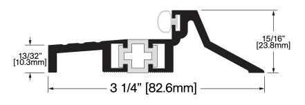
**Operation:** Thermal Break Threshold Features: Mill Finish Extruded Aluminum with Silicone Insert included Application: Ideal for Residential, Commercial & Industrial Maximum Length: 192 in [4877 mm]
