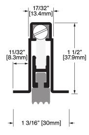
**Operation:** Automatic Door Bottom Features: Mill Finish Extruded Aluminum with Neoprene Maximum effective drop: 5/8 in (15.9mm) Application: Ideal for Residential, Commercial & Industrial
