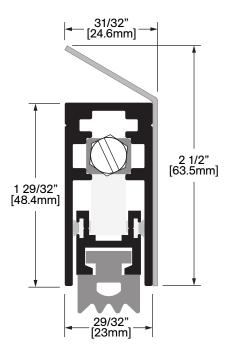
**Operation:** Automatic Door Bottom Features: 18 GA. 304 SS. 2B Stainless Steel Cover Clear Anodized Extruded Aluminum with Neoprene Maximum effective drop: 11/16 in (17.5mm) Application: Ideal for Residential, Commercial & Industrial
