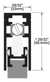
**Operation:** Automatic Door Bottom Features: Clear Anodized Extruded Aluminum with Felt Maximum effective drop: 11/16 in (17.5mm) Application: Ideal for Residential, Commercial & Industrial
