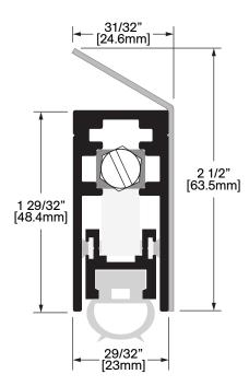
**Operation:** Automatic Door Bottom Features: 18 GA. 304 SS. 2B Stainless Steel Cover Clear Anodized Extruded Aluminum with Silicone Maximum effective drop: 11/16 in (17.5mm) Application: Ideal for Residential, Commercial & Industrial
