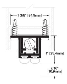
**Operation:** Automatic Door Bottom for Hollow Metal Doors Features: Mill Finish Extruded Aluminum with Silicone
