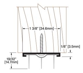
**Operation:** Door Shoe Features: Mill Finish Extruded Aluminum with Santoprene Co-Extrusion Application: Ideal for Residential, Commercial & Industrial Maximum Length: 144 in [3658 mm]
