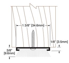
**Operation:** Door Shoe Features: Mill Finish Extruded Aluminum with Pile Application: Ideal for Residential, Commercial & Industrial Maximum Length: 150 in [3810 mm]
