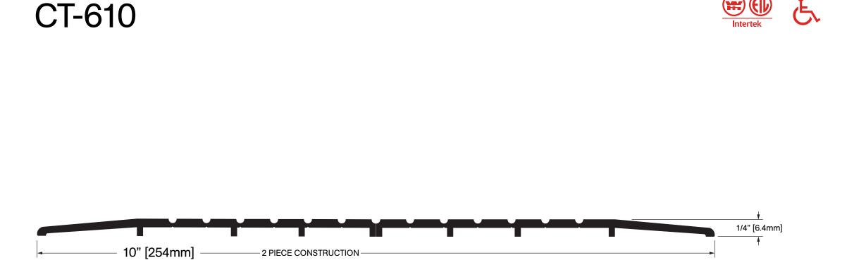
**Operation:** Threshold Features: Mill Finish Extruded Aluminum Application: Ideal for Residential, Commercial & Industrial Maximum Length: 156 in [3962 mm]
