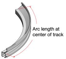
Radius to center of track/door, add 1 1/2 in [38.1 mm] to wall radius
