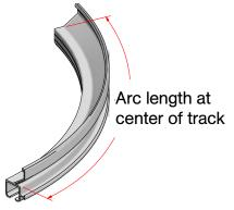
Radius to center of track/door, subtract 1 1/2 in [38.1 mm] to wall radius
