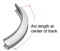
Radius to center of track/door, add 1 1/2 in [38.1 mm] to wall radius
