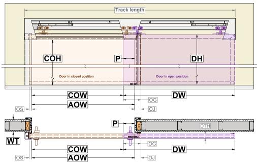
Maximum door size is 72 in [1829 mm] wide  $[DW] \times 120$  in [3048 mm] high  $[DH] \times 1$  3/4 in [45 mm] thick [TH], weighing up to 300 lbs [136 kg].
