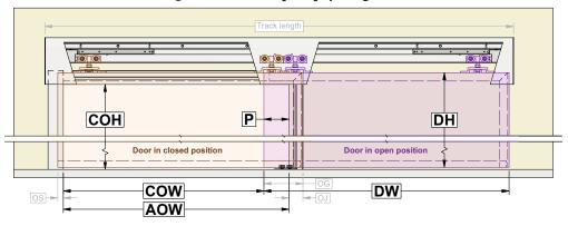
Maximum door size is 72 in [1829 mm] wide [DW] x 120 in [3048 mm] high [DH] x 1 3/4 in [45 mm] thick [TH], weighing up to 300 lbs [136 kg].
