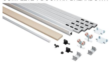
Each kit includes one CP-803 Header Track x length based on kit size, two CP-HB2X4 Header Brackets, two CP-830 Drywall Support x length based on kit size, four Steel Uprights x length based on kit size, two CP-2X4 Foot Brackets, two C-400 Hangers, two CDC-400 Catch/Stops, one C-201 Guide Channel x length based on kit size, one CP-200 Pocket Guide and necessary fasteners
