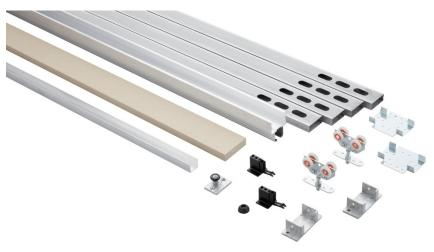
Each kit includes one CP-803 Header Track x length based on kit size, two CP-HB2X4 Header Brackets, two CP-830 Drywall Support x length based on kit size, four Steel Uprights x length based on kit size, two CP-2X4 Foot Brackets, two C-400 Hangers, two CDC-400 Catch/Stops, one C-914 Guide Channel x length based on kit size, one CP-913 Pocket Guide and necessary fasteners
