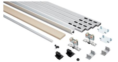
Each kit includes one CP-806 Header Track x length based on kit size, two CP-HB6MS Header Brackets, two CP-930 Drywall Support x length based on kit size, four (or six) Steel Uprights x length based on kit size, two (or three) CP-6MS Foot Brackets, two C-411 Quick Release Hangers, two CDC-411 Catch/Stops, one C-201 Guide Channel x length based on kit size, one CP-200 Pocket Guide and necessary fasteners.
