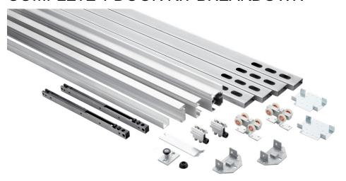
Each kit includes one CP-406 Header Track x length based on kit size, two CP-HB6MS Header Brackets, two CP-930 Drywall Support x length based on kit size, four Steel Uprights x length based on kit size, two CP-6MS Foot Brackets, two CC-493 Easy Connect Catch 'N' Close Hangers, two CC-100 Catch 'N' Close In-Track Stops, two Catch 'N' Close Closing Devices, one C-914 Guide Channel x length based on kit size, one CP-913 Pocket Guide and necessary fasteners.
