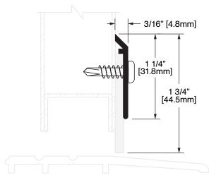
**Operation:** Door Sweep Features: Clear Anodized Extruded Aluminum with Grey P.V.C. Application: Ideal for Residential, Commercial & Industrial Maximum Length: 144 in [3658 mm]
