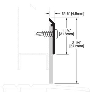
**Operation:** Door Sweep Features: Clear Anodized Extruded Aluminum with Black Solid Neoprene Application: Ideal for Residential, Commercial & Industrial Maximum Length: 144 in [3658 mm]
