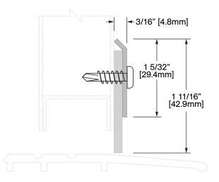
**Operation:** Door Sweep Features: Stainless Steel with Black Solid Neoprene Application: Ideal for Residential, Commercial & Industrial Maximum Length: 84 5/8 in [2150 mm]
