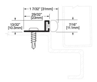
**Operation:** Weatherstrip Features: Clear Anodized Extruded Aluminum with Silicone Application: Ideal for Residential, Commercial & Industrial Maximum Length: 144 in [3658 mm]
