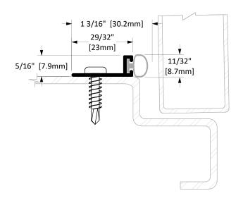
**Operation:** Weatherstrip Features: Clear Anodized Extruded Aluminum with Silicone Application: Ideal for Residential, Commercial & Industrial Maximum Length: 144 in [3658 mm]
