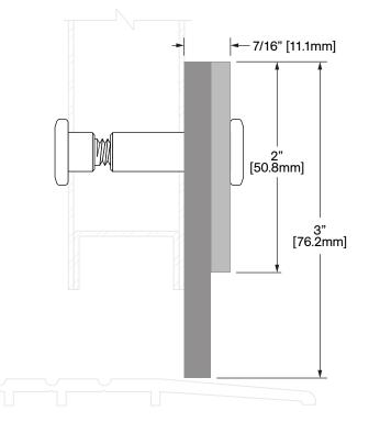
Operation: Heavy-Duty Door Sweep Features: Extruded Aluminum with 1/4 in [6.4 mm] Thick Solid Neoprene Application: Ideal for Residential, Commercial & Industrial Maximum Length: 144 in [3658 mm]
