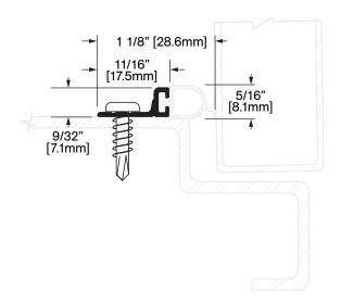
**Operation:** Weatherstrip Features: Mill Finish Extruded Aluminum with VInyl Fin Application: Ideal for Residential, Commercial & Industrial Maximum Length: 144 in [3658 mm]
