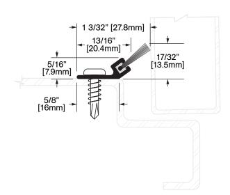
**Operation:** Weatherstrip Features: Clear Anodized Extruded Aluminum with Nylon Brush Application: Ideal for Residential, Commercial & Industrial Maximum Length: 120 in [3048 mm]
