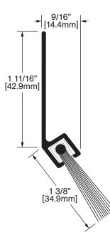
**Operation:** Door Sweep Features: Mill Finish 2 in Aluminum Angle with 1 in Nylon Brush Application: Ideal for Residential, Commercial & Industrial Maximum Length: 144 in [3658 mm]
