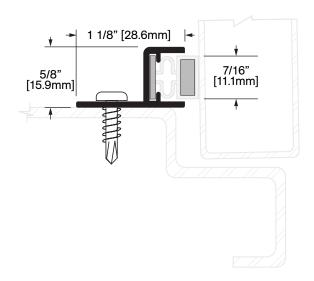
**Operation:** Weatherstrip Features: Clear Anodized Extruded Aluminum with Vinyl & Magnet Application: Ideal for Residential, Commercial & Industrial Maximum Length: 144 in [3658 mm]
