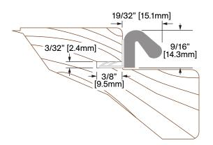
**Operation:** Kerf Mounted Weatherstrip Features: Seamless Santoprene Elastomeric Skin Seal Compressed size: 1/4 in Application: Ideal for Residential, Commercial & Industrial Maximum Length: 144 in [3658 mm]
