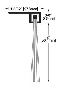
**Operation:** Door Sweep Features: Clear Anodized Extruded Aluminum with 2 in Nylon Brush Application: Ideal for Residential, Commercial & Industrial Maximum Length: 144 in [3658 mm]
